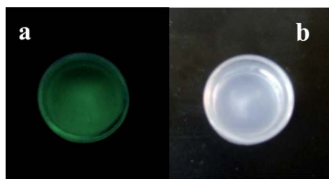
Fig. 14 Color of MDPCT (W) dissolved in n -hexane (a) under UV ( \lambda_{\text{ex}} = 250 nm), and (b) natural daylight.
